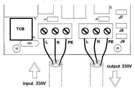
Figure 1: Input and output terminals
