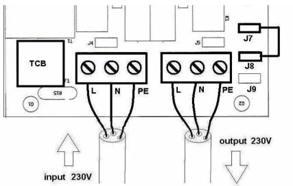
Figure 3: Output neutral grounding
