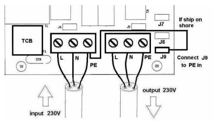
Figure 2: Input earth connection
